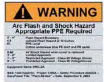
Figure 6 – Equipment Specific Field Label
