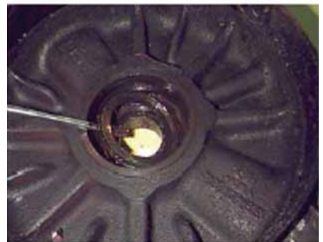
Figure 8. Shield was pressurized by excessive grease which caused a cage failure.
