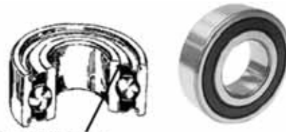
Seal wipes or slides against inner race
